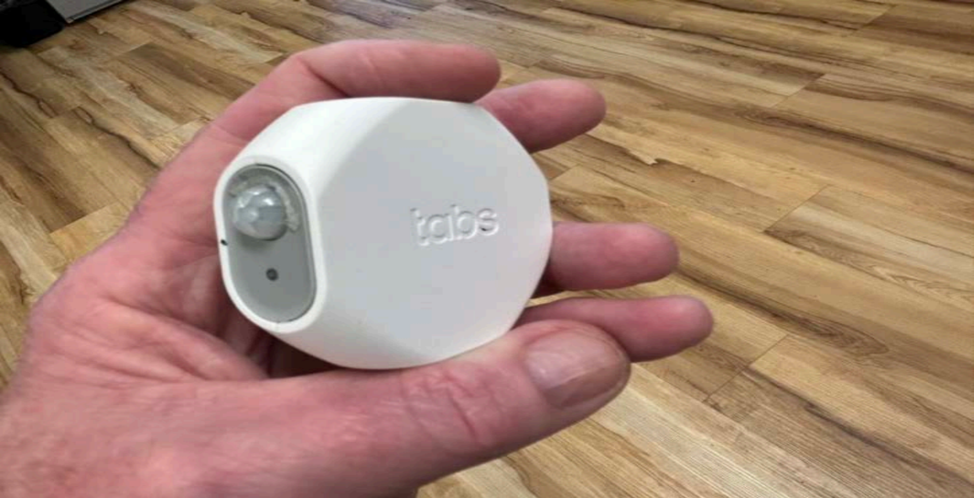
Figure 90. These small, powerful rodent sensors, can be placed inside exterior bait stations (toxic or non-toxic), or can be installed w/o bait box to monitor for the 24/7/365 presence or absence of rats (or mice inside) around or inside a property. Alerts of each rodent at each minute of a day/night and their precise location are sent to a phone, tablet or desk computer. Data dashboard software provide up-to-date alerts and status, and progress of rat control on blocks, alleys, parks, building perimeters, refuse staging corrals, campuses, and many other applications. Essential technology large-scale Rat IPM programs as well as for municipality program cost efficiency. (EverSmart® Rodent Sensors (Microshare.io) shown here, but no endorsement implied over any other rodent remote sensor technology).
