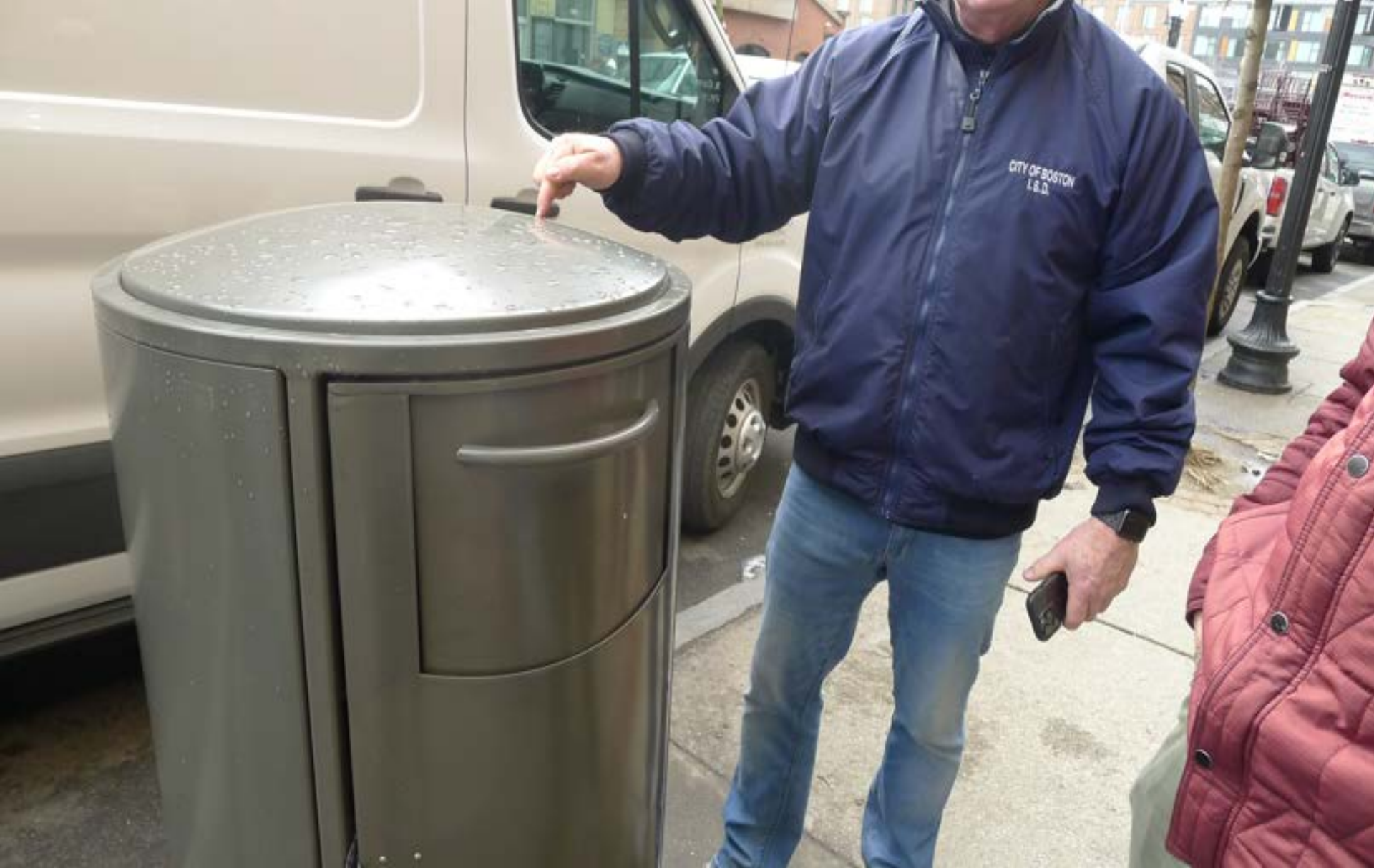
Figure 72. A new ‘rat-proof’ litter basket is being piloted in Boston. The key to its sustainability will be the hatch door staying in good condition to prevent the can from getting jammed open due to overfilling.
